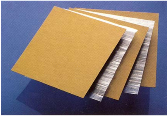
Fig. 1 Composition of a GLARE 2-3/2-0.4 laminate
